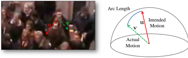
Fig. 1. Pedestrian efficiency in videos can be defined by the difference between the intended and actual motions represented with 3D optical flow vectors. Left: The intended direction \mathbf{u} of an individual may be inhibited causing them to move in a different direction \mathbf{v} . Right: We measure the difference between these motions with arc-length on the unit sphere, which is inversely proportional to efficiency.
