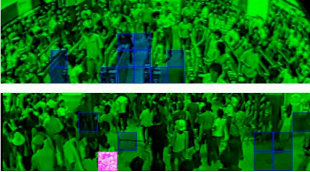
Figure 8. Areas lacking in pedestrian motion that usually contain it are successfully detected in both data sets. False positives indicate a sensitivity to unusual textures.
